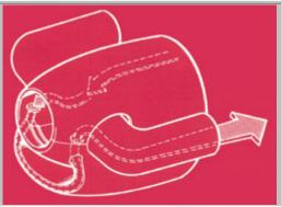
In the original configuration, hot exhaust gas is extracted from both exhaust stacks and is ducted down both sides of the intake lip, to heat the lip and them exits out the bottom of the cowling just aft of the lip.
